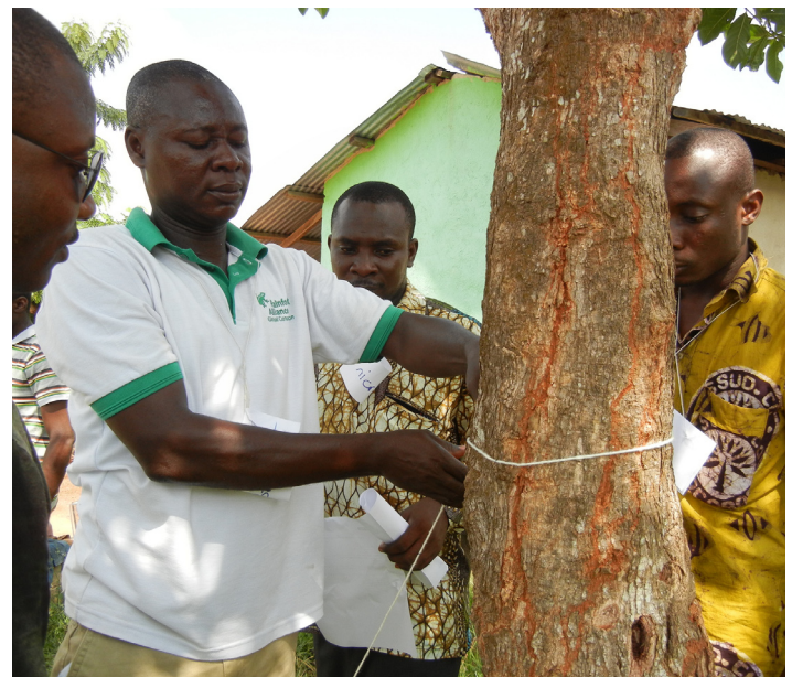
Rainforest Alliance staff at a teacher training in Ghana demonstrate how to measure a tree to calculate the amount of carbon it contains.
